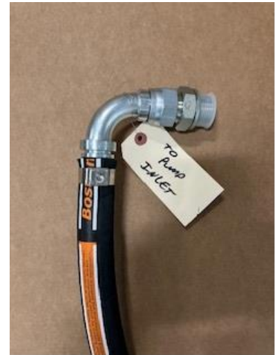
Fig. 8: Install 90° radius hose to pump inlet.
