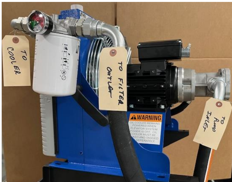
Fig. 9: Complete heat exchanger with filter head and two hoses.
