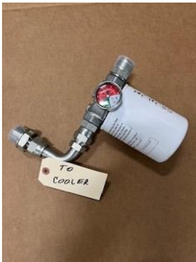
Fig. 6: Install 90° radius filter head to heat exchanger.
