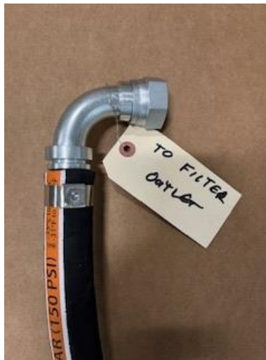
Fig. 7: Install 90° radius hose to filter head outlet.
